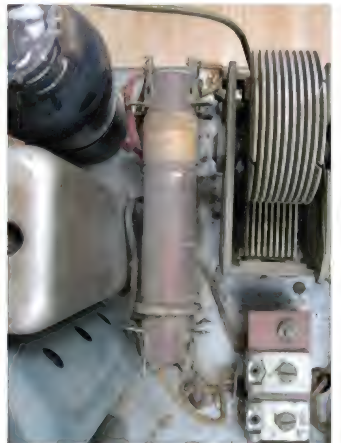
The other two oscillator coils sharing a common coil form on top of the chassis.
